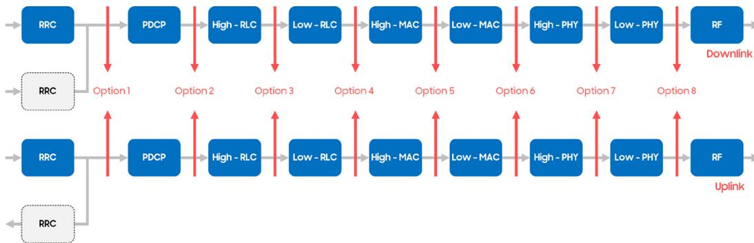
Figure 7 : Radio Access Functional Split
