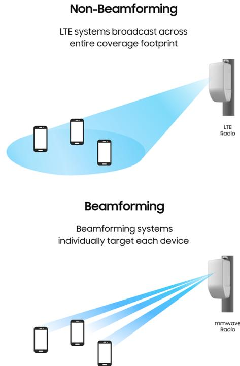
Figure 3: Traditional antenna radiation vs. Beamforming
